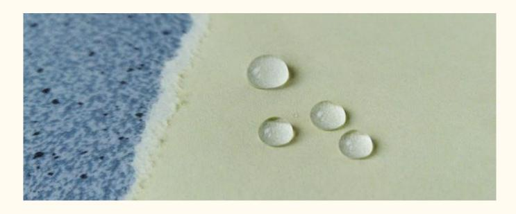
Hybrid bio-based materials: mechanical and functional properties of cellulosic substrate coated with ceramic by atomic layer deposition
