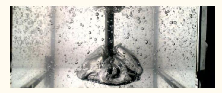
Hydrodynamics of a pneumatic agitator for methanisation processes
