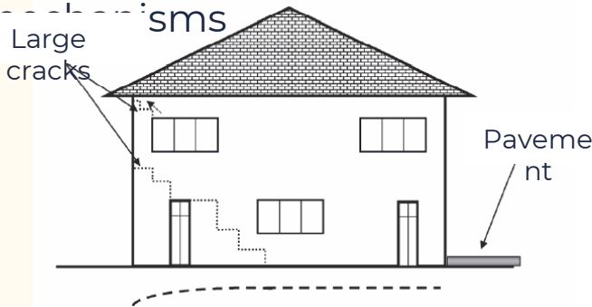
Deformation mode caused by peripheral shrinkage of the soil under the house
